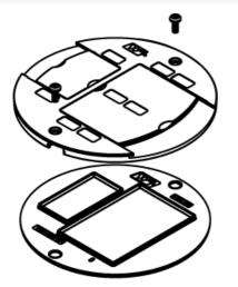
Nonmetallic slide holder assembly. Available in gray (GY), black (BK), ivory (VY), aluminum colored (AL) and brass colored (BS). NOTE: Assembled with scrub water gasket. For use on tile or carpet floors. AMD8 Series Poke-Thru Devices require a 4" (102mm) diameter hole. Not designed to work with bare concrete or terrazzo. Floor covering thickness 1/8" minimum.
