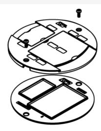
Nonmetallic slide holder assembly. Available in gray (GY), black (BK), ivory (VY), aluminum colored (AL) and brass colored (BS). NOTE: Assembled with scrub water gasket. For use on tile or carpet floors. AMD8 Series Poke-Thru Devices require a 4" (102mm) diameter hole. Not designed to work with bare concrete or terrazzo. Floor covering thickness 1/8" minimum.
