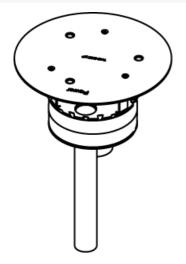
Use with AMD8C Series Covers to complete installation. AMD8 Series Poke-Thru Devices require a 4'' (102mm) diameter hole. Not designed to work with bare concrete or terrazzo. Floor covering thickness 1/8'' minimum.
