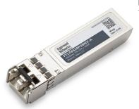
Finisar FTLF8528P2BNV Compatible 10GBase-SR SFP+ Transceiver (MMF, 850nm, 300m, LC Duplex, DDM, I-Temp)
