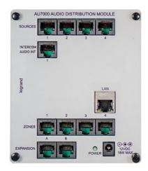
The Audio Distribution Module is used to connect up to four sources to the On-Q Digital Audio System and distribute those sources to four zone outputs. It can be expanded to accommodate up to sixteen sources and sixteen zo
