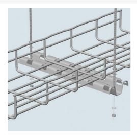
Designed to take the place of traditional strut in a trapeze application. Our FAS Profile system attaches to tray with no nuts or bolts. It is a safer, faster option to install suspended wire mesh cable tray. Can be cut to the length required for installation.
