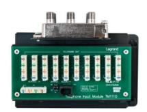
The 10x8 combo distributes up to four telephone lines to ten network locations, and one digital video line to eight locations from a cable company approved Antronix splitter. This module also provides RJ31X line seizure port for home security system configuration.
