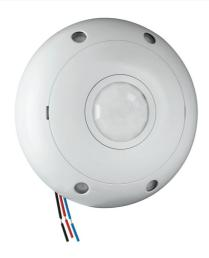
The sensor shall detect occupancy in the control area by detecting Doppler shifts in transmitted ultrasound and passive infrared heat changes. Detection verification of both technologies must occur in order to activate lighting systems. Upon verification, detection by either shall hold lighting on.
