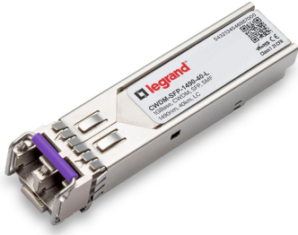
Cisco CWDM-SFP-1490-40 Compatible 1000Base-CWDM SFP Transceiver (SMF, 1490nm, 40km, LC Duplex, DDM, I-Temp)
