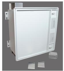
12" deep termination block enclosure for 2'  $\times$  2' drop ceiling tile. One removable mounting plate for two 300 pair 1100 style termination blocks (without legs).
