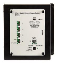
This versatile triple-speed Ethernet interface can operate as either a 4-port Gigabit Broadband Router or a 5-port Gigabit Switch, selectable with the flip of a switch. In Router mode, it scapable of up-linking with virtually any ADSL or Cable modem,
