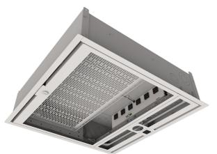
Fully finished enclosure designed to manage and store A/V equipment in an air handling plenum space above a NO ceiling. Has a built-in projector mount that utilizes a 1 1/2" standard NFS fitting and is rated to support a load up to 50 lbs. The projector mount can move laterally and be positioned anywhere along the track.
