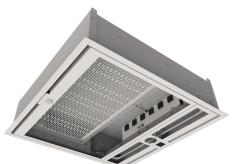
Fully finished enclosure designed to manage and store A/V equipment in an air handling plenum space above a NO or hard ceiling. These boxes are also equipped with the <u>RackLink system</u>, <u>by Middle Atlantic Products</u>. The box also has a built in projector mount that utilizes a 1 1/2" standard NFS fitting and is rated to support a load up to 50 lbs. The projector mount can move laterally and be positioned anywhere along the track.
