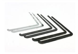
Used for floor coverings greater than 3/6" (4.7mm). The EFB45-TS allows the finished cover assembly to be flush with the finished floor. Includes one (1) 1/16" (1.6mm), one (1) 1/8" (3.2mm) and one (1) 1/4" (6.4mm) tile shims for 7/16" (11.1mm) of upward adjustment.
