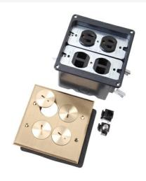
Tamper-Resistant Floor Box Assembly, Dual-voltage. Two #8 duplex openings, Four threaded screw plugs. Includes 3232 15A, 125A tamper-resistant duplex receptacle, Cat5E Jack, F-connector, Ten Blanks and a low-voltage dider. Brass. For detailed Tamper-Resistant receptacle information, visit our Tamper-Resistant Receptacles page.
