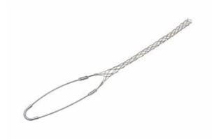
Stainless Steel, Standard-duty, Closed Mesh, Single eye grip. Cable Diameter -.0500-.0610\'\', Bale length, 7\'\', Mesh length, 11\'\', Break strength, 770 lbs.
