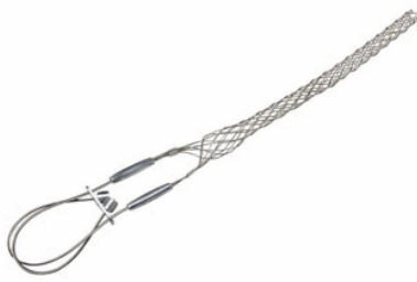
FC062LB: Standard Duty, Closed Mesh, Locking Bale (Universal Eye), Cable Diameter 0.62 - 0.74 inches, Bale Length 18-in, Mesh Length 11-in, Break Strength 1150 lbs.
