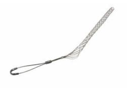
Stainless Steel, Standard-duty, Closed mesh, Offset eye grips. Cable diameter -0.750-0.990\'\', Bale length - 4\'\', Mesh length - 14\'\', Break strength - 960 lbs.
