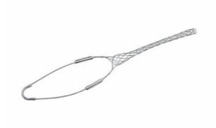
Stainless Steel, Standard-duty, Closed mesh, Single eye grips. Cable Diameter -1.750-1.990\'\', Bale length - 14\'\', Mesh length - 20\'\', Break strength - 2,640
