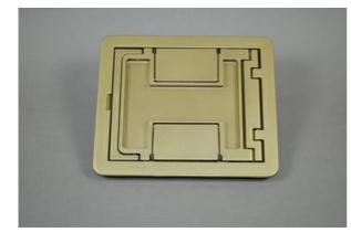
Flanged cover for use in tile or carpet installation. Die-cast aluminum assembly. Lid area is flush with the finished floor, no cutouts provided. TR indicates tamper-resistant version secured with tamper-resistant screw. North American made.
