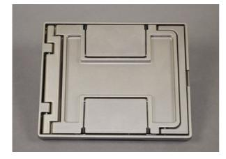
Flangeless cover for use in tile installation. Die-cast aluminum assembly. Insert in lid allows for tile cutouts to match finished floor. NOTE: Add suffix "TR" to the end of the part number to indicate tamper-resistant cover assembly. Tamper-resistant versions are secured with a single tamper-resistant screw.
