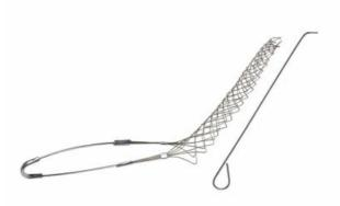
Stainless Steel, Standard-duty, Split rod, Single eye. Cable diameter - 0.620-0.740\\', Bale length - 8\\', Mesh length - 11\\', Break Strength - 960 lbs.
