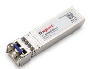
Finisar FTLX1472M3BCL Compatible 10GBase-LR SFP+ Transceiver (SMF, 1310nm, 10km, LC Duplex, DDM, I-Temp)
