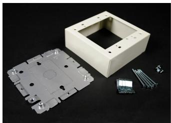
Two Gang Device Box. Cover has twistouts for 2000, 500 and 700 Series Raceways. Base has 1/2" trade size KO and rectangular KO for extension to wall box. Base has #10 threaded hole for ground connection.
