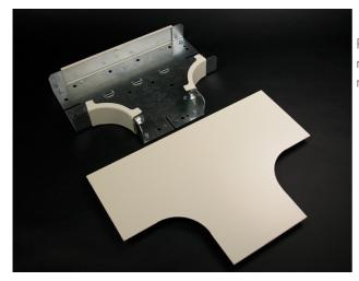
Full capacity, undivided tee fitting. Provides 2" (51mm) cable bend radius control for UTP, STP and fiber optic installations. Ideal for new installations whether the cable is lay-in or pull-through.
