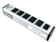
Five 250V, IEC 320 outlets, gray finish, 10A single pole circuit breaker, power cord not included. Length 11' (279mm). Receptacle center-to-center 1 1/2'' (38mm). Input is provided with a male IEC320 Receptacle. Appropriate input cord must be purchased separately. Output receptacles are female IEC320. Snap-on, slide-off mounting. Power cord not included. NOTE: cULus Listed, TUV Nord Certified EN0950.
