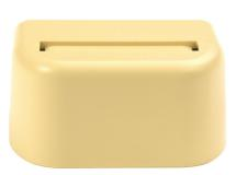
TechChoice surface mount boxes accept 2 rear loading keystione jacks & modules and provides easy snap-on covers and snap-in label fields. Boxes are supplied with screws and double-sided adhesive tape for mounting onto almost any surface. Meet UL2043 and are suitable for installation in air handling spaces (ie plenum spaces) and are compatible with Wiremold Eclipse raceway.
