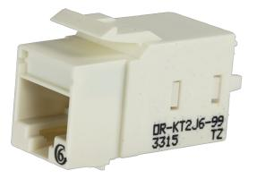
Category 6 Keystone jack, 8-position, 180 degree exit, icon compatible, T568A/B wiring, Fog White , individually packaged.Keystone, KT2J jacks and modules feature New installer friendly lacing cap termination with free termination tool in every carton. The keystone footprint allows flexibility in installation scheduling because its rear insertion into the faceplate allows the technician to complete the termination before and during the construction process.
