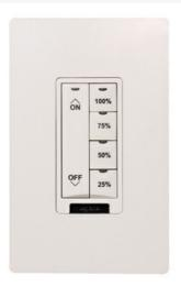
LMDW-100 Series Digital Dual Technology Wall Switch Occupancy Sensors use PIR and ultrasonic technology to detect occupancy for energy-efficient control of lighting and plug loads. They also include one or two switch buttons for manual control of selected loads, and are part of a Wattstopper Digital Lighting Management (DLM) system.
