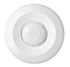
The LMPC-600 wireless low profile Digital PIR Ceiling Mount Occupancy Sensor uses passive infrared (PIR) technology and one of three lenses to detect occupancy in different types of spaces for energy-efficient control of lighting and plug loads. It is a digital sensor, and is part of the NEW wireless Wattstopper Digital Lighting Management (DLM) system.
