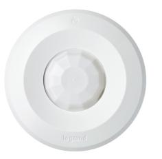
The LMPC-600 wireless low profile Digital PIR Ceiling Mount Occupancy Sensor uses passive infrared (PIR) technology and one of three lenses to detect occupancy in different types of spaces for energy-efficient control of lighting and plug loads. It is a digital sensor, and is part of the NEW wireless Wattstopper Digital Lighting Management (DLM) system.
