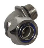
Rated IP68 and NEMA 4X, Stainless Steel Liquid-Tight Connectors offer corrosion resistance for the toughest environments. For use in wet or dry locations to seal electrical connections against dust, dirt, oil, water, chemicals and other corrosive elements. These are available in straight and 90 degree, 3/8"" to 2"" NPT. The stainless steel liquid-tight offering includes a nylon-insulated throat and Viton O-Ring.
