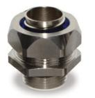
Rated IP68 and NEMA 4X, Stainless Steel Liquid-Tight Connectors offer corrosion resistance for the toughest environments. For use in wet or dry locations to seal electrical connections against dust, dirt, oil, water, chemicals and other corrosive elements. These are available in straight and 90 degree, 3/8"" to 2"" NPT. The stainless steel liquid-tight offering includes a nylon-insulated throat and Viton O-Ring.
