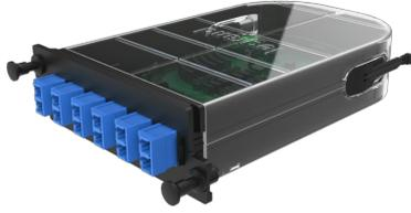
The 12 fiber cassettes support fusion splicing of individual fibers, while the 24 fiber cassettes support fusion splicing of ribbon fibers. Heat shrinks, pigtail slack and cable slack are managed within the cassette—eliminating the need for individual splice trays or housings. The design of the cassettes allows easy mounting from either the front or the rear of an enclosure or panel, and individual fibers within the cassette may be accessed without disturbing the other fibers in the housing.
