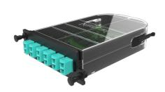
Infinium Quantum Splice Cassettes are available in the Infinium M4 footprint, enabling industry leading performance, fast field termination, and providing cable management within the housing. The Splice Cassettes are designed for use with Single-Mode (OS2) or Multimode (OM4/OM5) Fiber, Houses 12-24 fibers and are available in LC Duplex or LC Quad port configurations.
