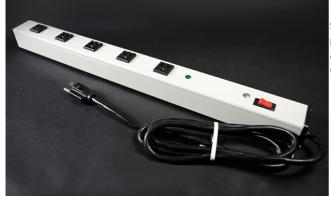
Sentrex high performance surge protection. Five outlets, lighted switch, durable putty white aluminum housing, 15A. Receptacles rotated 90 degrees and spaced to accommodate transformers. Length 24"" (610mm). 6' (1.8m) 14/3 SJT putty white cord with NEMA5-15 plug. Snap-on, slide-off mounting.
