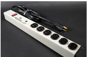
Perma Power computer grade surge protection. Six outlets, lighted switch, durable putty white aluminum housing, 20A. 6' (1.8m) 12/3 SJT putty white cord with NEMA 5-20 plug. Length 18"" (457mm). Snap-on, slide-off mounting.
