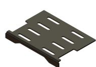
Zero rack unit horizontal managers slide into the slots in the Mighty Mo 20 fingers and provide support for fiber and copper cables exiting horizontal equipment modules. They toollessly lock into place with the 19" version mounting between 2 vertical managers in front of the equipment. Internal versions are sized to fit inside the vertical managers and provide a continuous horizontal path across the front of the racks and managers.
