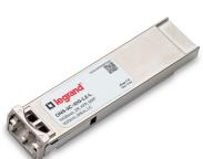
Cisco ONS-XC-10G-L2 Compatible 10GBase-ZR XFP Transceiver (SMF, 1550nm, 80km, LC Duplex, DDM, I-Temp)
