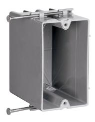
This single-gang, deep switch and outlet box features captive mounting nails, threaded mounting holes, and two quick entries on each end. Durable and impact-resistant, this thermoplastic box contains innovative extras that cuts installation time. Extra deep for dimmers, GFCIs and thermostats, yet suitable for 2x4 construction. Qty 100
