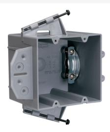
Range or Dryer Box with captive Mounting Screws on Each End. 1/2inch offset for wood or steel stud mounting with metal cable clamp. 12 pack.
