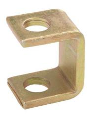
Use closed clips with 1-1/2 in stringers to secure runway to threaded rods when suspending runway from the ceiling. Also use when stacking runway. Use with 5/8 in-11 in threaded rod. Made of 1/4 in x 1-1/2 in steel bar. UL classified.
