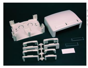
Surface mount box for use with Eclipse Raceway or standalone application. Has two 1/2'' trade size KOs. Accepts two front-loaded downward facing Pass and Seymour Activate or Wiremold Open System communication modules.
