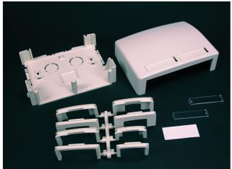
Surface mount box for use with Eclipse Raceway or standalone application. Has two 1/2" trade size KOs. Accepts two front-loaded downward facing Pass and Seymour Activate or Wiremold Open System communication modules.
