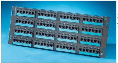
Clarity 6 96-port high density Category 6 patch panel is component compliant to EIA/TIA Category 6 performance requirements. It occupies four rack units and measures 19" x 7". Jacks are grouped in six-port modules. Part of the Clarity 6 link and channel solution that provides significant installed performance headroom.
