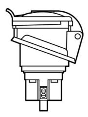
Triple-Pole, 4-Wire, Receptacle. 16A, 200/250V.
