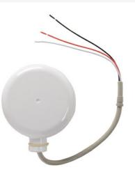
PIR High Bay Wet Fixture Sensor, 120/277 VAC, 60hz, Coverage 60 ft. diameter @ 40 ft. mounting height.
