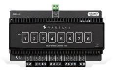
The Relay Station Lighting - DIN is designed to control lights and provides eight isolated latching relay channels. The RS8-L-DIN accepts voltage from 0 to 277 volts and up to 10amps at each load. The relays are single-pole, single throw, offering a set of eight latching contacts. This station may also be used as a low-voltage relay station. Actuator buttons allow the connected relays to be manually toggled. Relays latch in place retaining its last state in case of a power interrupt.
