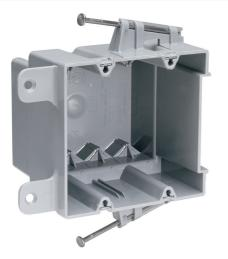
Double Gang Switch and Outlet Box with captive mounting nails on each end and four auto alamps on each end. It is easy toinstall with a rectangular cutout. It is durable and hasanimpact-resistant thermoplastic box. It contains innovative extras that cut installation time. 50 pack
