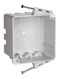
4-inch Square Box with Threaded Mounting Holes, captive Mounting Nail each end. Three Auto/Clamps each end, Two on side adjacent to nails. Two #8 mounting screws factory installed.
