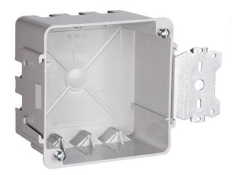
4-inch Square Box with Threaded Mounting Holes for Wood and Steel Stud Mounting. Three Auto/Clamps each end, Two on side opposite bracket. Two #8 mounting screws factory installed.
